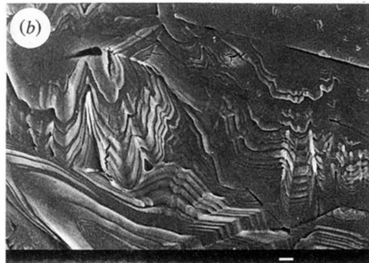
Figure 18. Powdered d\text{-LiKC}_4\text{H}_4\text{O}_6\cdot\text{H}_2\text{O} after dehydration ( \alpha = 1.00 at 463 K). Textures of product salt are similar to those found in single crystals dehydrated at relatively higher temperatures (figure 10 a , b ). There is evidence of extensive sintering of the recrystallized outer surface. (Scale bar: ( a ) 100 \mu\text{m} ; ( b ) 1.0 \mu\text{m} .)
